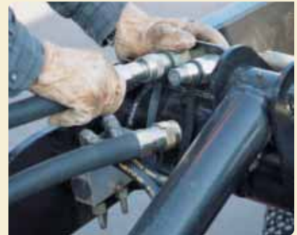
3) For powered attachment, connect hydraulic lines to dripless flush-face quick couplers on loader arms.
