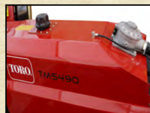
Large oil reservoir for efficient cooling.
