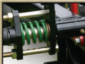
Wing unit spring to minimise collision damage.
