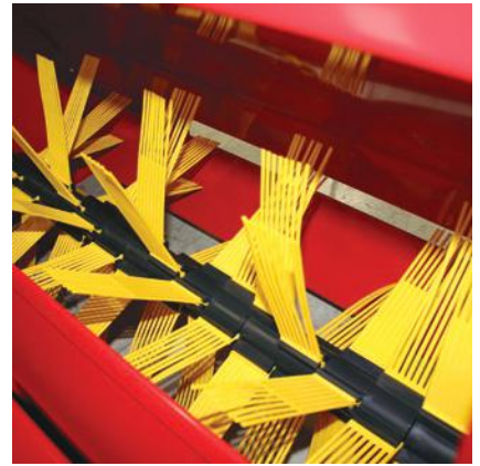
The Powered Grass Collector uses brushes to sweep up the grass cuttings
