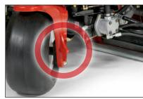
Jack points on all three wheels make removal of front and rear tires a breeze, and fluid sight levels on hydraulic and fuel tanks make daily visual maintenance checks fast and easy.
