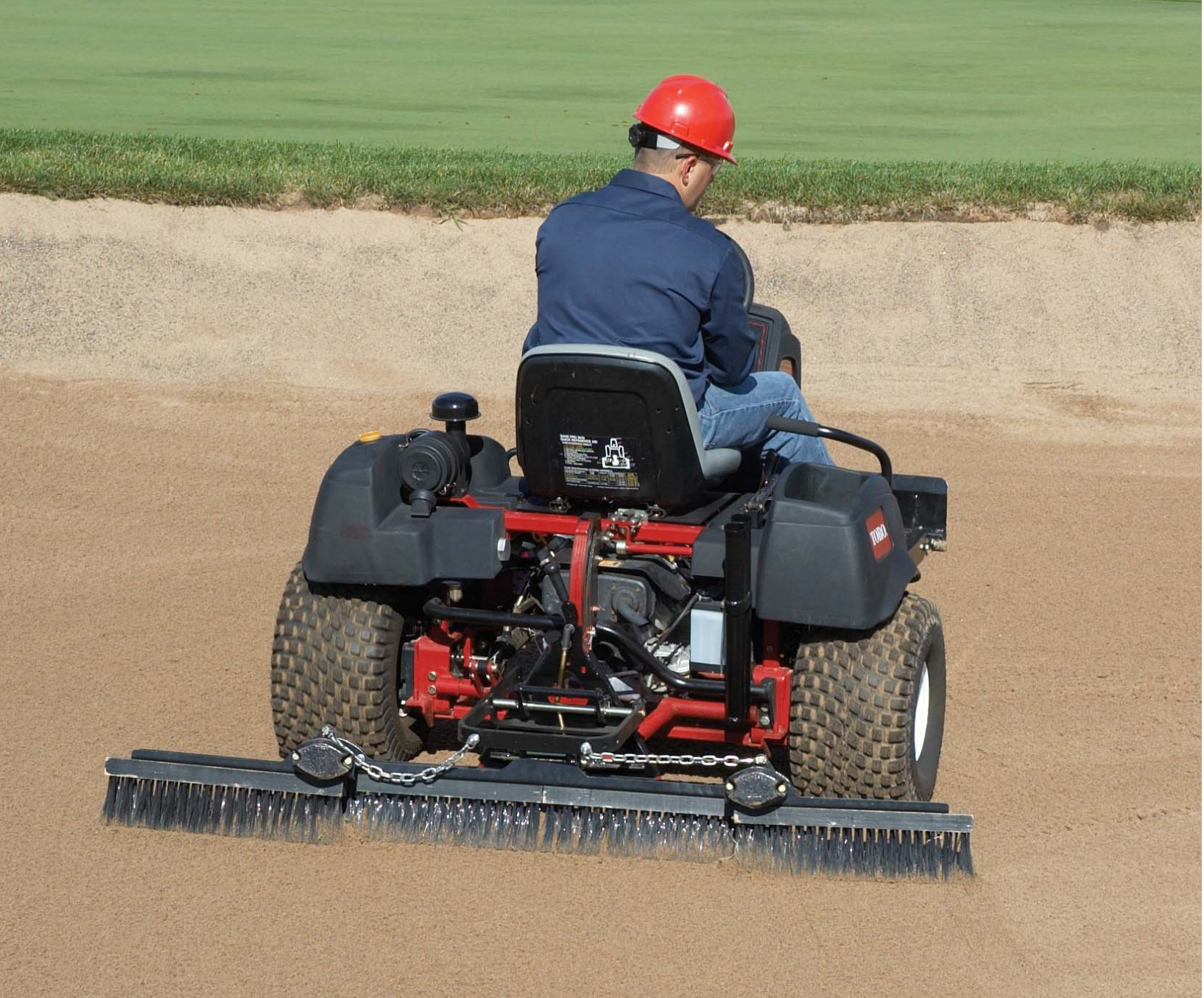
The segmented grooming broom attachment smoothes and shapes without fluffing.
