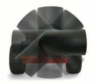
Operators can also use the wireless remote control to rotate the nozzle a full 360 degrees in either direction, or adjust the engine throttle up or down to match air power to the job at hand.
