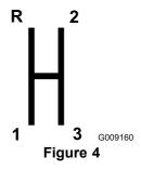
**Important:** Do not shift the transaxle to the reverse or forward gear unless the vehicle is standing still. Damage to the transaxle may occur.
