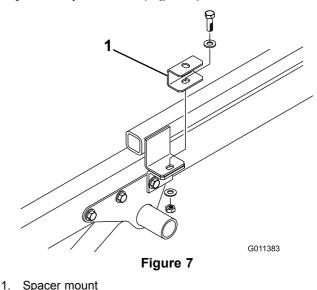
5. Position TopDresser onto vehicle frame, aligning holes in rear mounting brackets with holes in each side of frame (Fig. 7).
