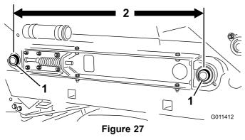
1. Conveyor belt roller shafts
