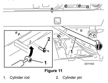
**Important:** Always unlock the dump stop lever before attempting to attach the cylinder for tilting. Use the tilt of the cylinders only for service of the engine or hydraulics underneath.
