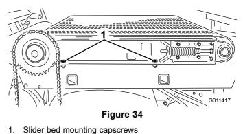
7. Remove (2) capscrews, washers and nut, on left side of machine, securing slider bed to frame (Figure 35).
