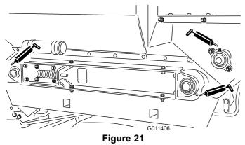
side to side. The brush adjustment should be checked weekly for wear. The bristles of the brush will wear under normal conditions and the distance from the brush to conveyor belt should be maintained to prevent uneven wear of the brush.
