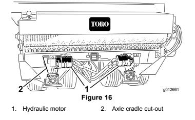
2. Rotate motor sprocket assembly until proper chain tension is attained.
