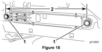
1. Conveyor belt roller shafts 2. 35-1/4 inches (895 mm)
