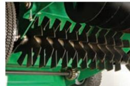
The seed rate control allows for seeding at variable rates and for different grass varieties and applications.
