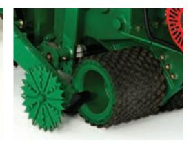
A forward metering wheel measures accurate sod cut lengths.
