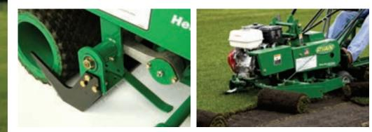
SOD HOLD DOWN SKIDS KIT The Sod Hold Down Kit keeps the sod from buckling and may be necessary in very sandy soil conditions or when the ground is dry.
