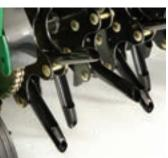
0.75-inch (19mm) diameter coring tines are made of hardened alloy steel for durability.
