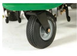
A unique front caster wheel allows the machine to maneuver with near zero-turn capability.
