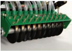
The curved shape of the discs direct the seed into the soil slits for ultimate seed-to-soil contact and maximum germination.
