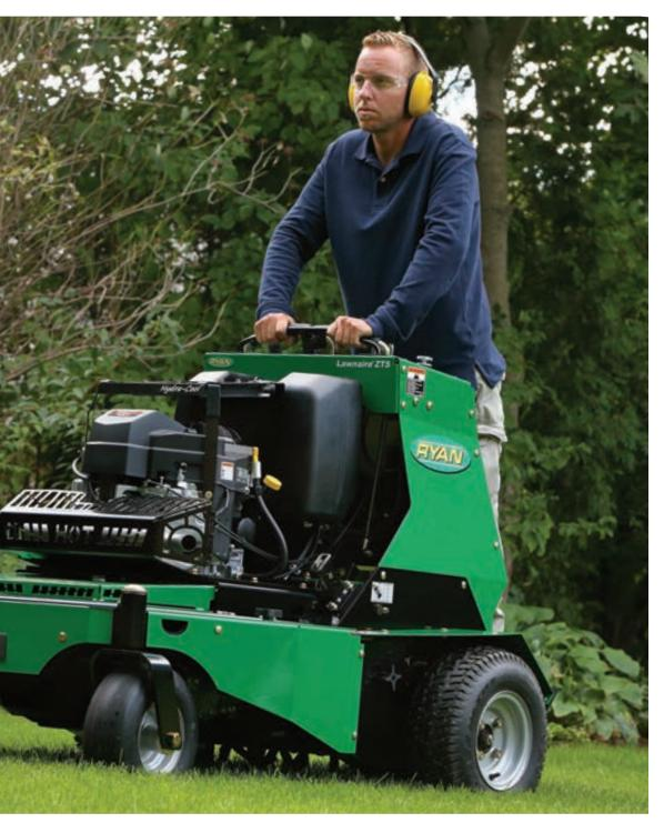
The intuitive control panel features a hydraulic pressure gauge with easy-to-read dial for management of down pressure under various
