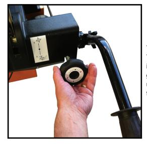
The blades must be **CLEAR** of the ground before adjustment commences. The depth of cut is adjusted by varying the height of the front rollers, using the micro adjuster. Start the engine and allow to warm up. Engage the ground wheel and reel drives and lower the reel using the micro adjuster until the required amount of thatch is being removed. Always disengage the reel drive when the machine is stationary on the green.
