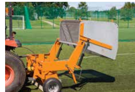
Hydraulic tip facility for easy emptying
