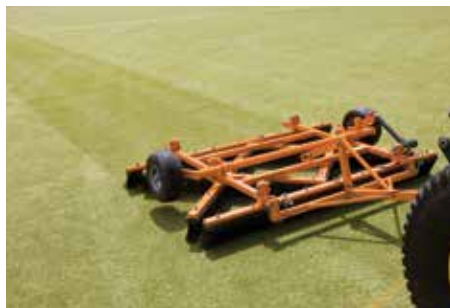
In action standing up the pile and moving the infill
