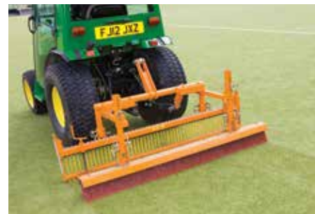
Twinplay with flexicomb and straight brush reducing compaction on sand infill
