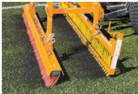
Stiffer bristles – Flexicomb crossbar set low for rubber crumb infill
