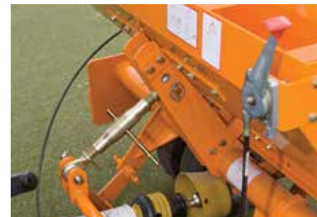
Cable control for material shut off
