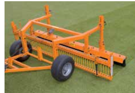
Towed frame with flexicomb and straight brush in action on sand infill
