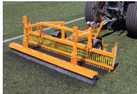
Towed frame with flexicomb and straight brush. The crossbar is low stiffening the bristles for rubber infill
