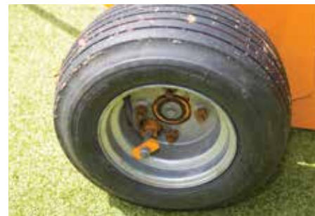
Simple “pull & twist” clutch levers on each wheel to disengage wheel drive to the brush during transport
