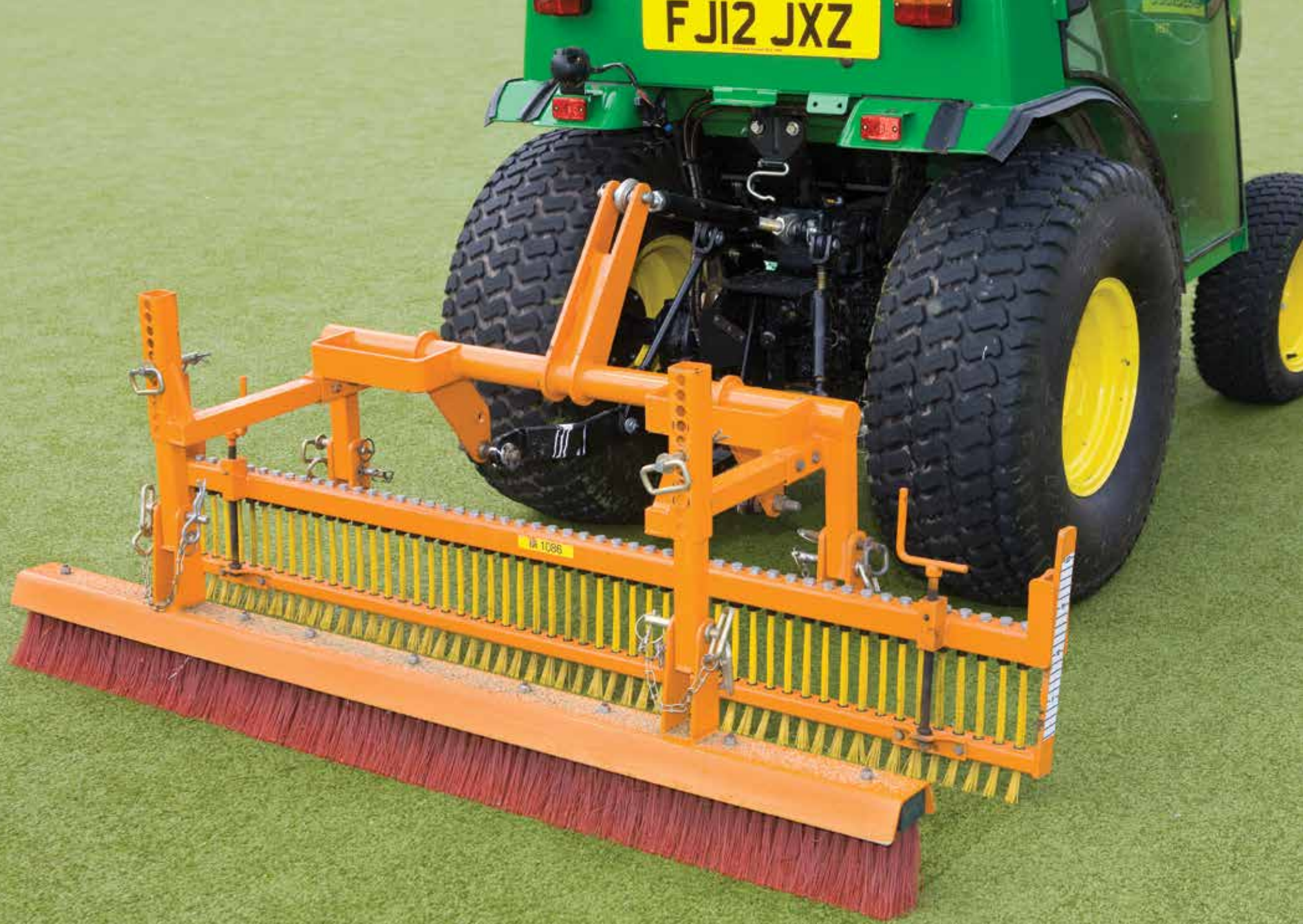
IMAGE SHOWS TWINPLAY FRAME WITH FLEXICOMB AND STRAIGHT BRUSH
