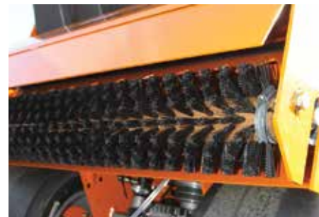
Powered rear discharge brush for even spread of material
