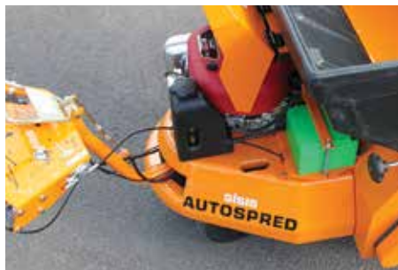
Simple pivot steer to access even the tightest corners
