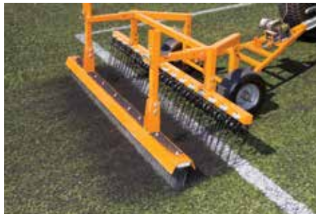
Towed frame with fine grooming rake and straight brush in action reducing compaction on rubber infill
