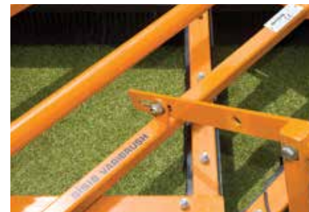
Adjustable drawbar for towing height
