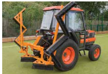
Outer sections fold hydraulically for transport and storage
