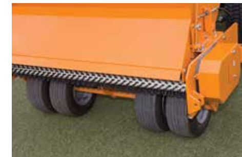
Four wheel axle gives even weight
