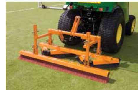
Zig Zag brush and straight brush combination at work on sand infill
