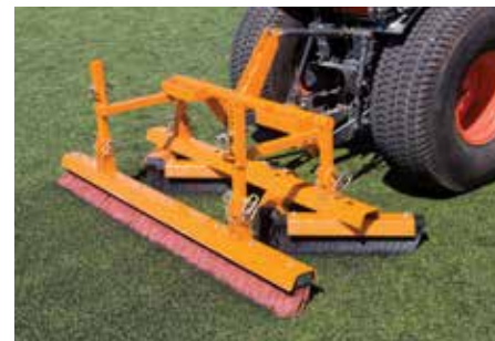
Zig Zag brush and straight brush combination at work on rubber crumb infill
