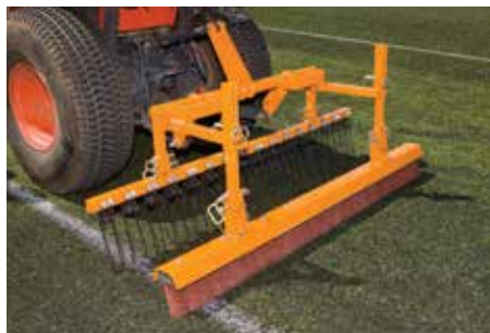
Twinplay with fine grooming rake and straight brush in action reducing compaction on rubber infill
