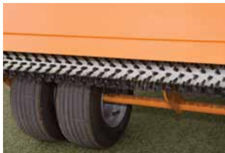
Rotating brush at point of discharge ensures even spread
