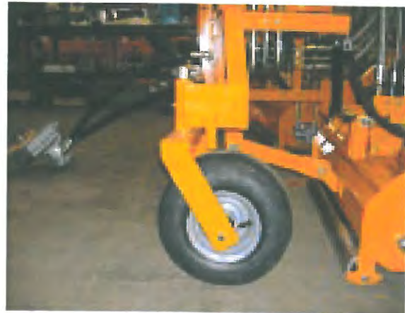
Figure 2 Assemble wheels by inserting shaft through casting. Secure wheel in place by securing top bearing with grub screw. Check for free movement
