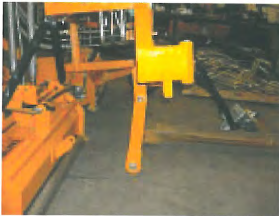
Figure 1 Showing pivot point for main wheels (one each side)
