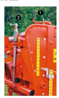
Achieve different spiking intensities by adjusting the tine entry angle.
